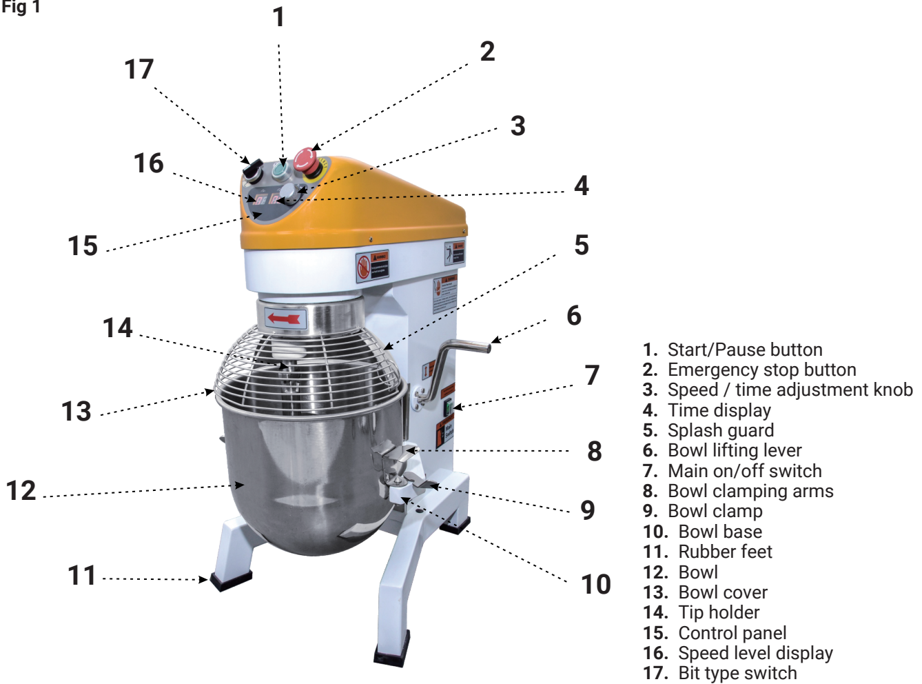
Figure 1 Construction of the device
