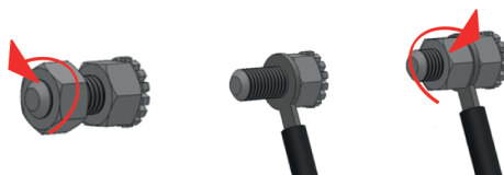
Figure 6. Connecting the unit to an electrical equalizing system.
