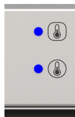
Fig. 12 Indicator light for chamber and boiler heaters
