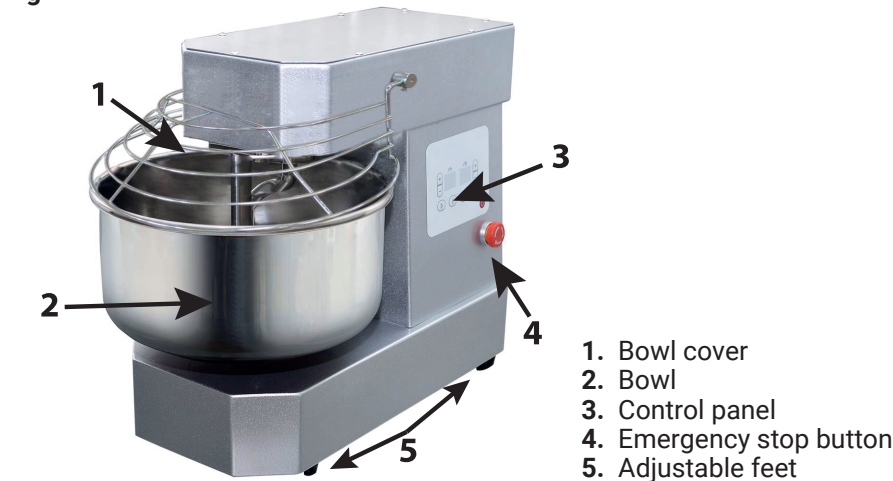
Figure 1 Construction of the device
